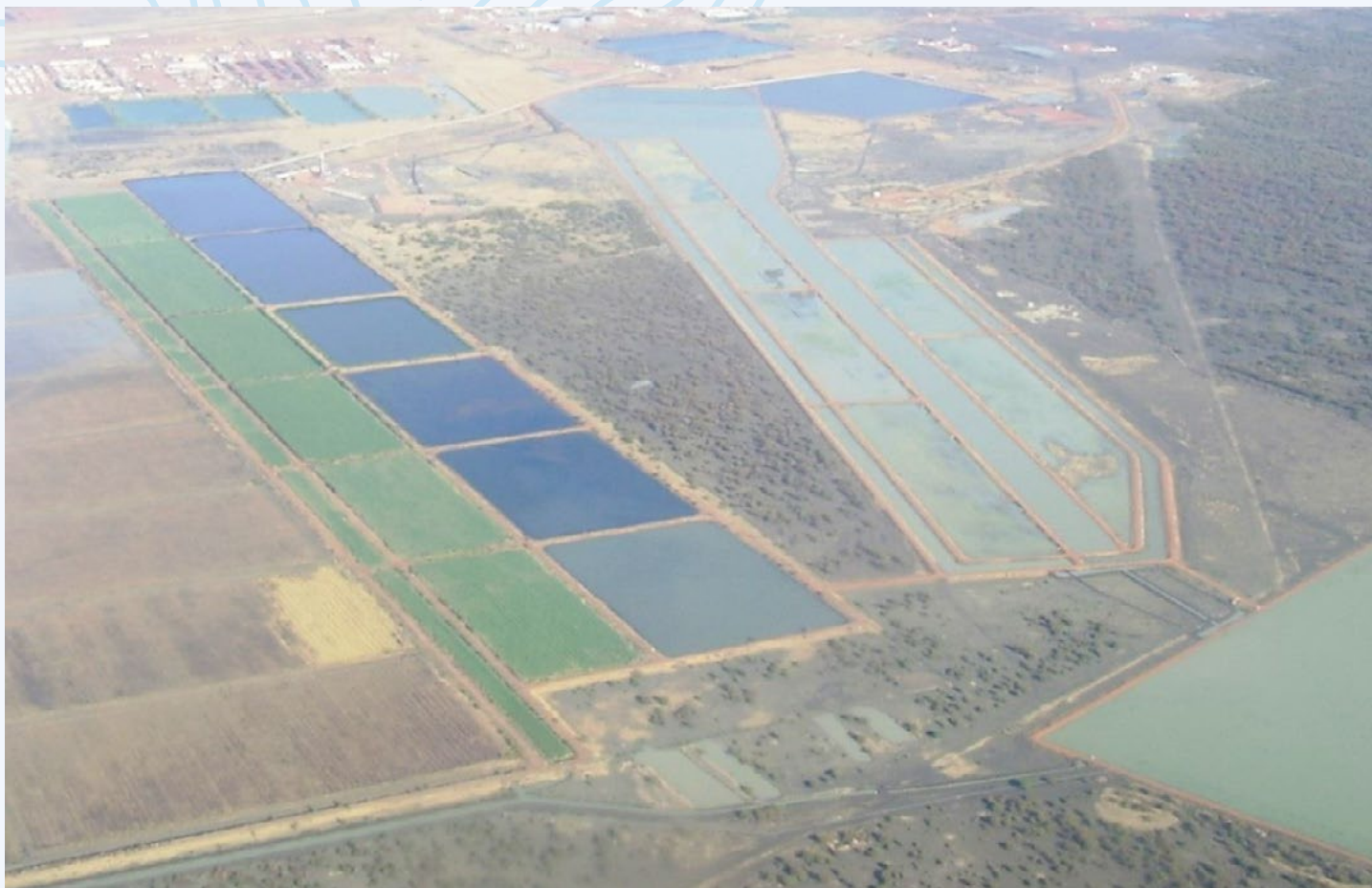
Photo 5. Bioremediation facility with settling lagoons and engineered wetlands (Heglig, Sudan)
